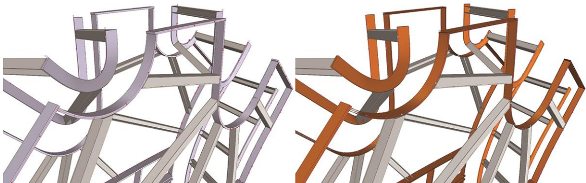
Figure 22. Double curved rail geometry before exporting to individual models (used courtesy of the authors with permission)
