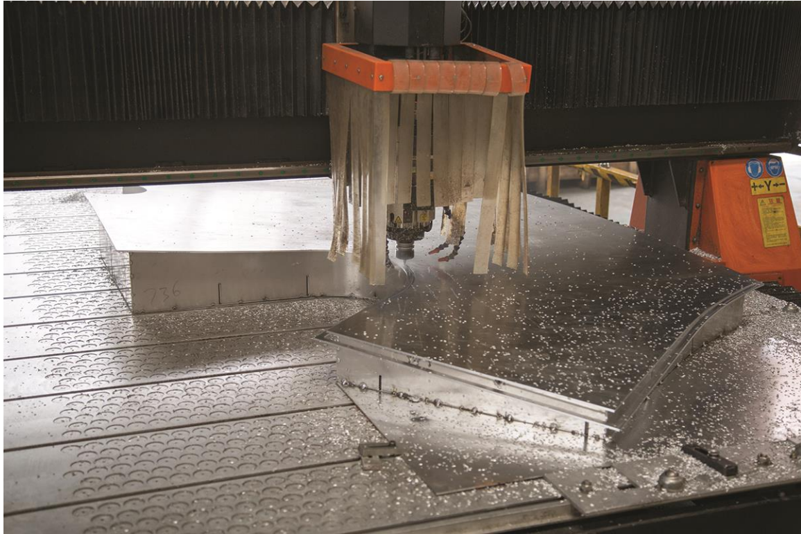
Figure 14. A post formed CNC cut panel, one part of one of the methods used to fabricate the exterior cladding panels
